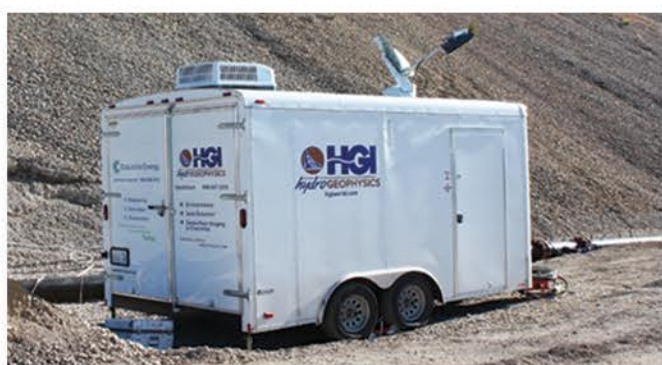
HGI's Geotection Resistivity Monitoring System deployed at a dam site
